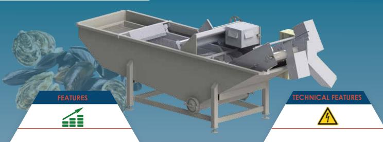
Oysters and other shellfish are sorted through different layered gratings using an eccentric mechanism.
